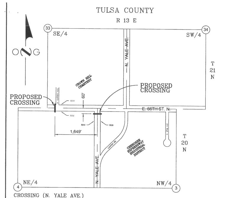
\* 2 3/8"OD API-5L, ERW, X-52, 3.66#, .154" WT PIPE INSIDE R/W 6 5/8"OD ASTM D2513 PE2406, 4.717#, .576"WT PLASTIC PIPE OUTSIDE R/W
